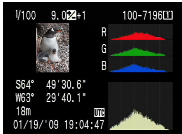
Figure 4: GPS co-ordinates stored with a digital photograph ( www.sjphoto.com/gps-canon.html )
